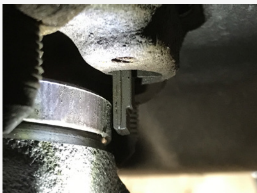
Fig. 2 Brake disc and sensor correctly installed
