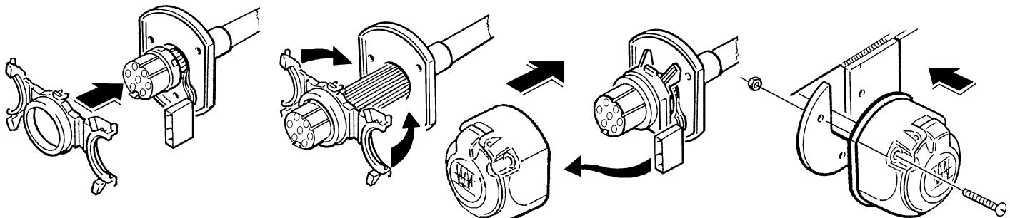
Put the harness's rubber bushing into place and slot it into the bushing of the jack compartment.
