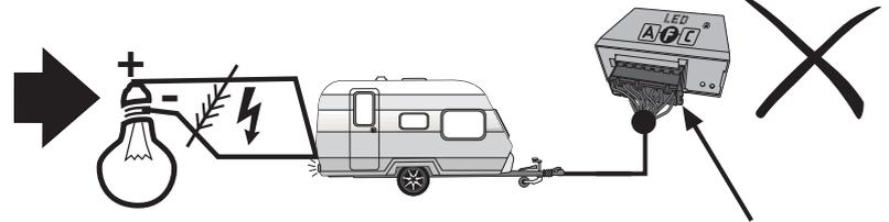
**Kurzschluss/Short circuit fault on PIN 7, 8 oder/or 10**
