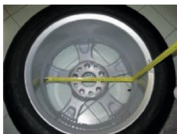
Figure F3.3.1. 1 Example of manual measuring of the external diameter (da2) of the wheel in the ALS1/ALS2 Programme Type
