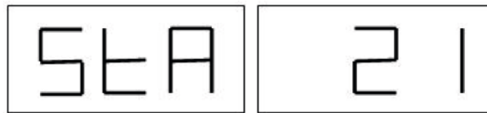
Fig. F8.1 View of the Static imbalance display enabled. The right display indicates the entity of the static imbalance.
